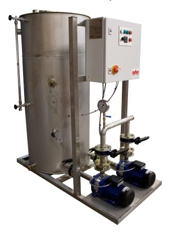
The Arbe range of ACR condensate recovery packages offer a compact solution for the collection of condensate from various systems. The product range offers a solution with the capability of handling up to 10,000 kg/hour of condensate as a standalone package. The tank, pumps and pipework are all manufactured from stainless steel and are designed for a long life.
