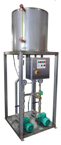
The Arbe range of ACR-N condensate recovery packages offer a reduced-footprint, compact solution for the collection of condensate from various systems. The unit has been designed to offer a solution where floor space or condensate operating height is critical, so the condensate tank is located over the pumps and controls.
